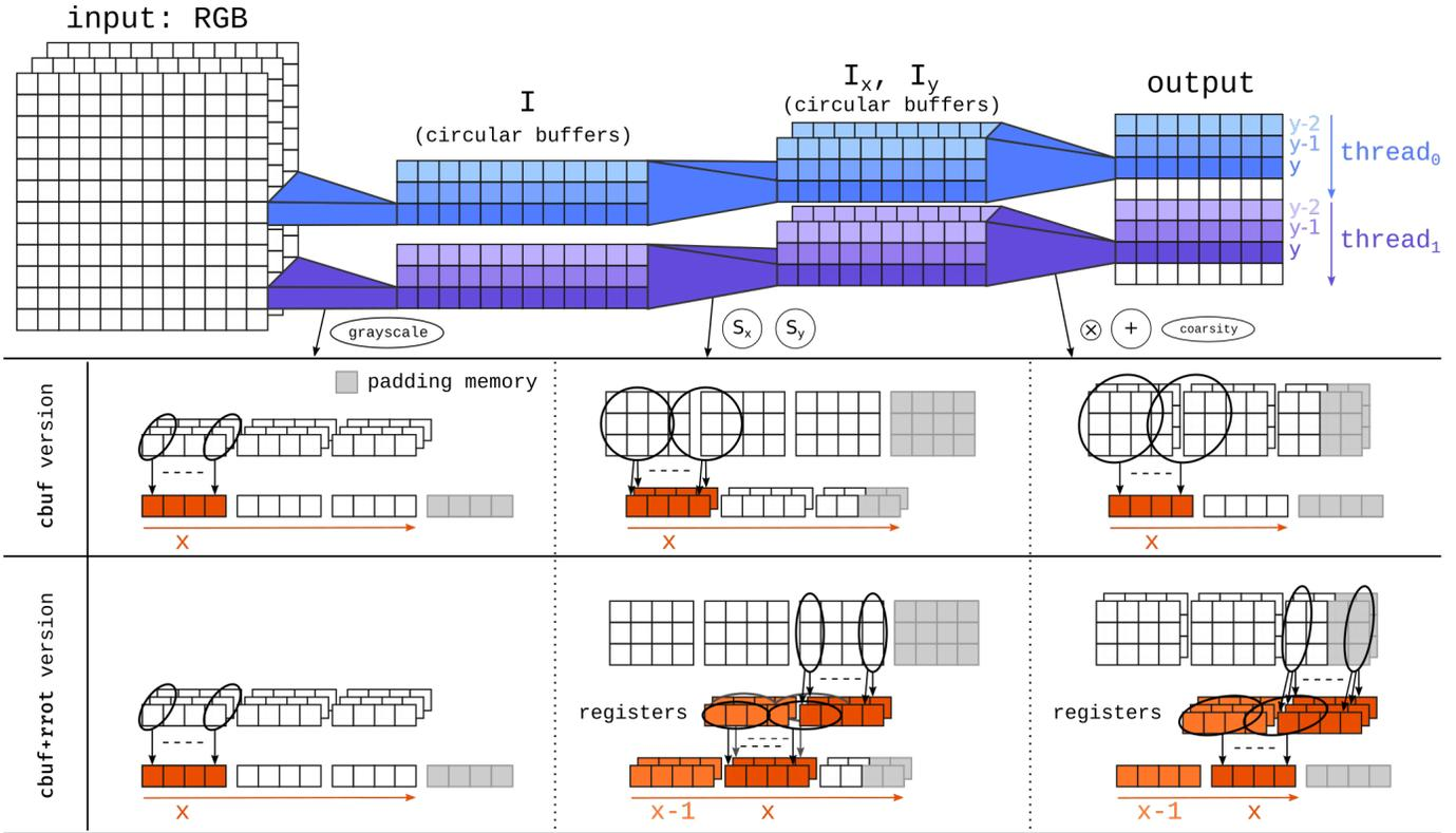
Fig. 6: Overview of the optimizations applied on the Harris corner detector.
