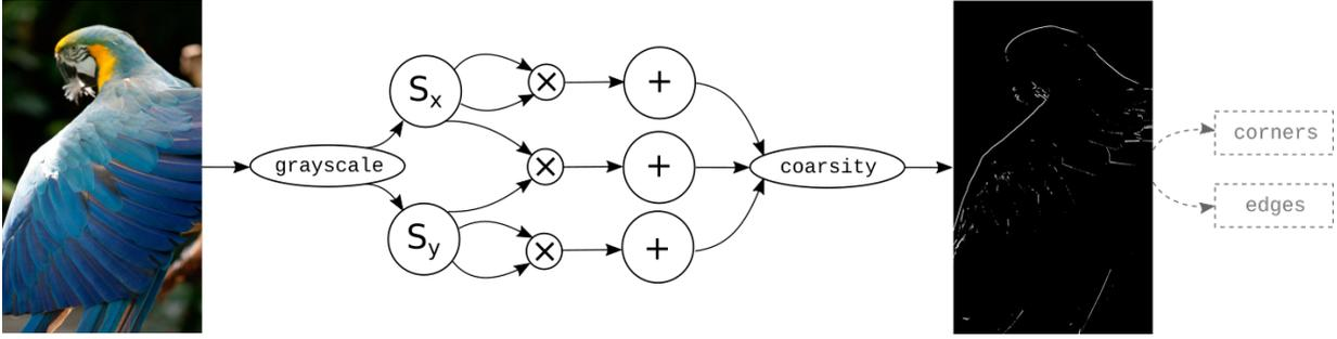
Fig. 5: Harris corner detection computation flow, illustrated with an example image from the Halide repository.
