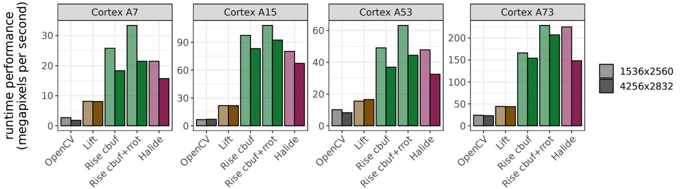
Fig. 8: Runtime performance of the Harris operator for the different processors, implementations and image resolutions.
