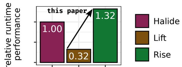
Fig. 1: The existing domain-extensible compiler LIFT performs poorly compared to Halide on image processing pipelines. Extended with additional optimizations, described as compositions of rewrite rules, our domain-extensible compiler for RISE outperforms Halide by 1.3× on Cortex A53.
