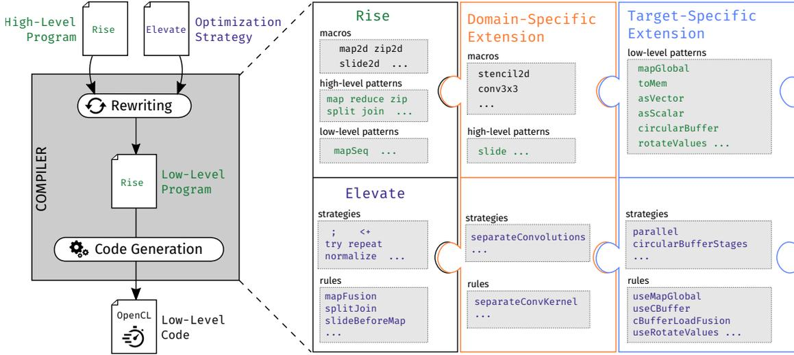
Fig. 2: A Domain-Extensible Compiler Design: Computations are expressed as compositions of extensible patterns in the RISE IR; Optimizations are expressed as compositions of extensible rewrite rules in the ELEVATE strategy language.
