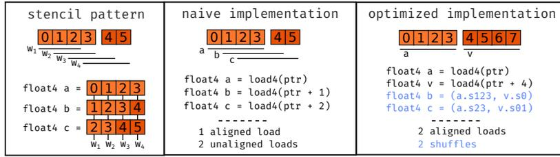
Fig. 7: Example of memory loads for a vectorized 1D stencil of size 3. The code is written in pseudo OpenCL syntax.
