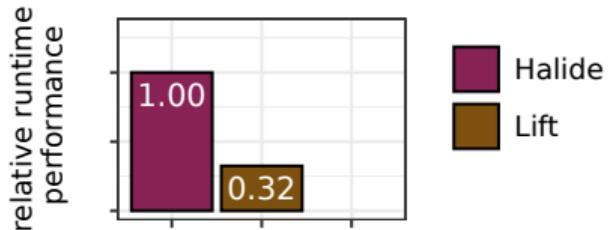
*LIFT performs poorly compared to Halide when compiling image processing pipelines, it is missing important optimizations.*
