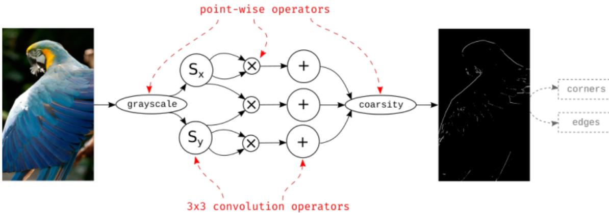
The Harris corner (and edge) detector is a well established image processing pipeline
